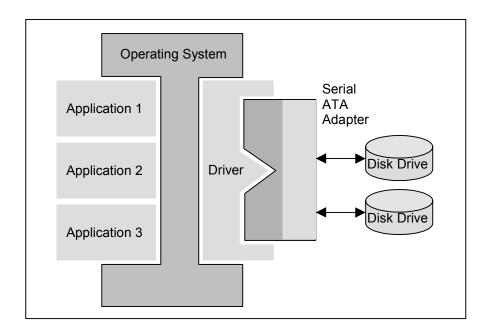
Figure 2.2 Drive system configuration
